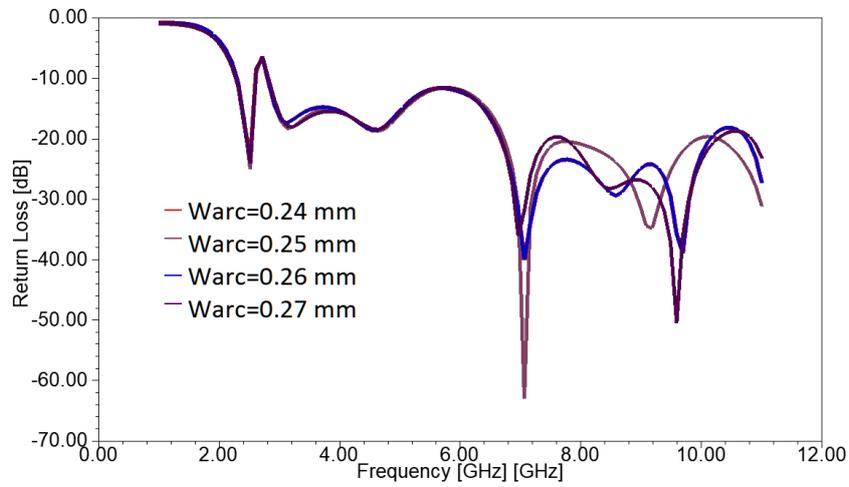
Fig. 6: Return loss plots for various arc widths
