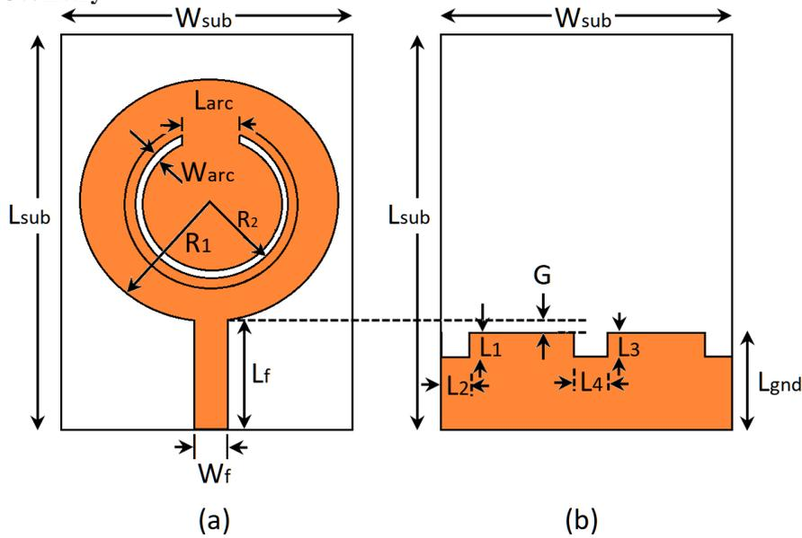
Fig. 3: Schematic of the proposed printed monopole Antenna with arc shaped slot.
