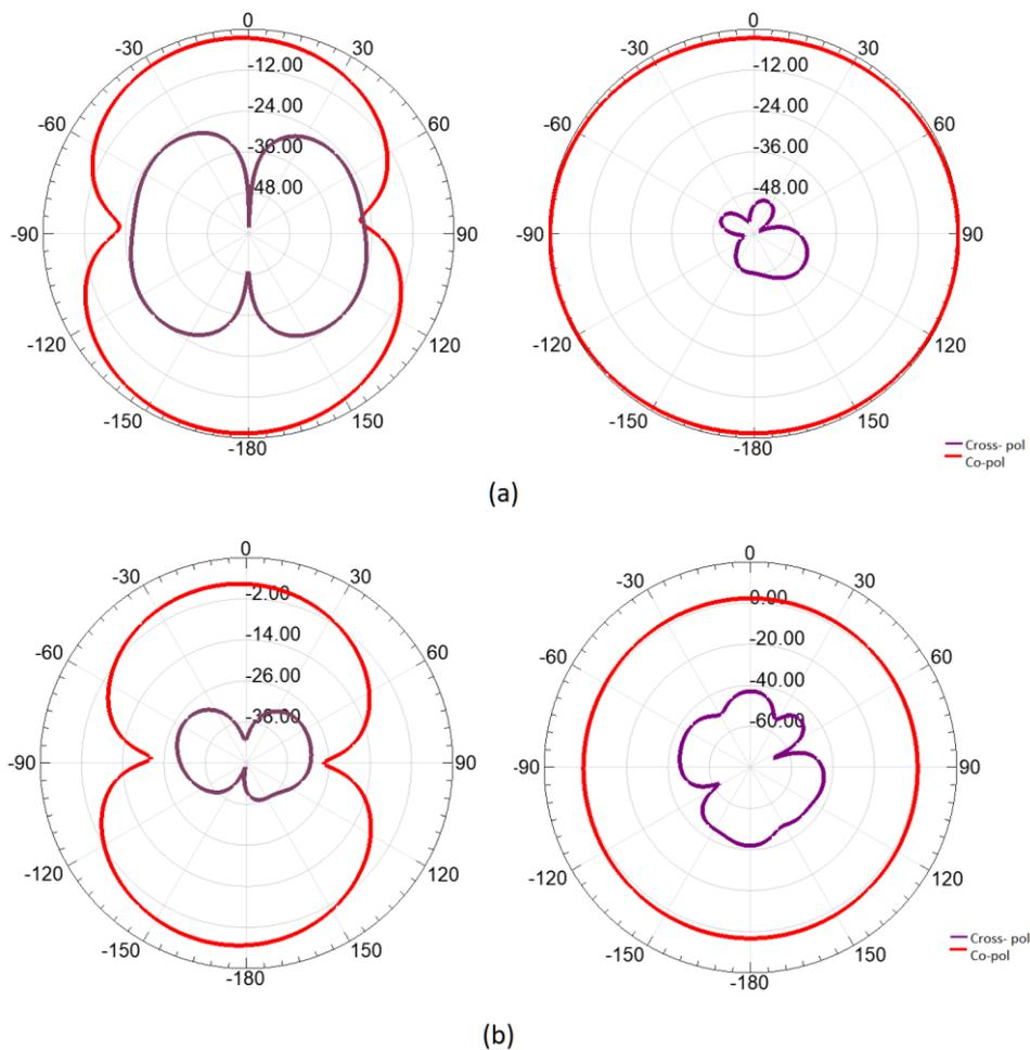
Fig. 9: E – Plane and H – Plane Radiation patterns at (a) 2.4 GHz, (b) 3.5 GHz.
