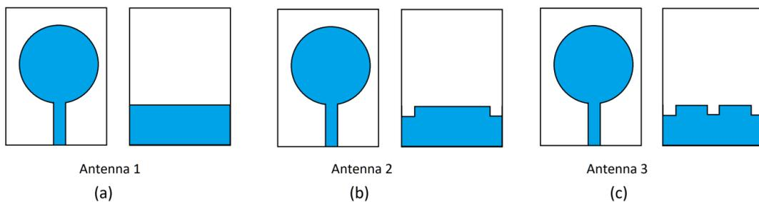
Fig. 1: The Evolution of printed circular shaped UWB monopole antenna.
