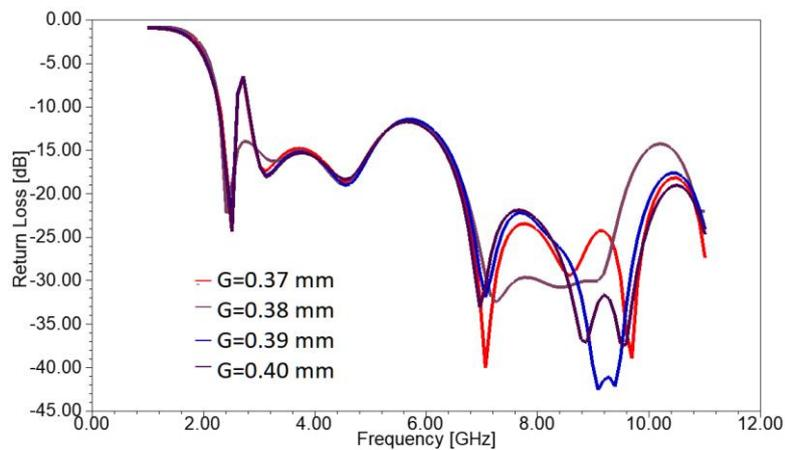
Fig. 7: Return loss plots for various gaps (G)
