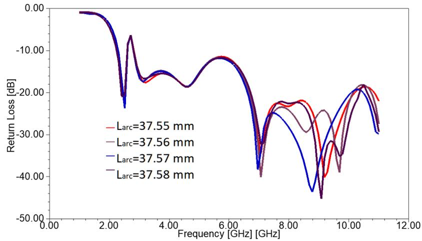
Fig. 5: Return loss plots for various arc lengths
