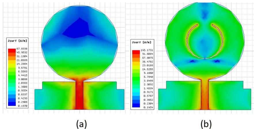
Fig. 4: Current distribution of the UWB antenna at 2.44 GHz; (a) without arc slots, (b) with slots.
